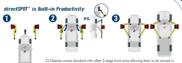
CLIUseries comes standard with ottset 3-stage front arms allowing them to be stowed in an asymmetric lifting position, rear of the front tires. Unlike many competitor lifts, when the vehicle is driven through, the front arms are capable of **directSPOT**<sup>™</sup> to the vehicle's lifting point without having to reposition the vehicle or shuffle back and forth to reach its recommended lift points.
