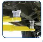
Optional **† 10318** frame engaging truck adapters can be used with 3" or 6" adapters. Simply take out the screw pad and drop in the stack extension and frame engaging adapter.
